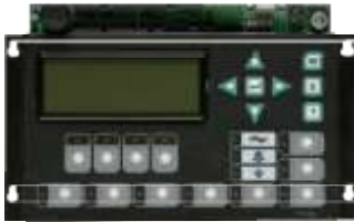
NK-AN-LCD large 80 character (4x20) back-lit LCD display
